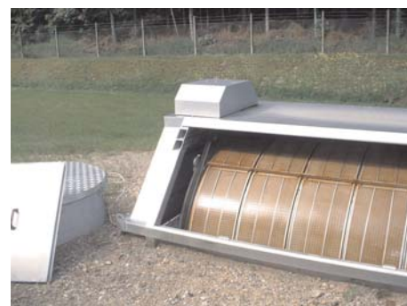
Picture: Phosphates are precipitated using iron-chloride and it can be seen that the filter cloth is becoming red in colour.
